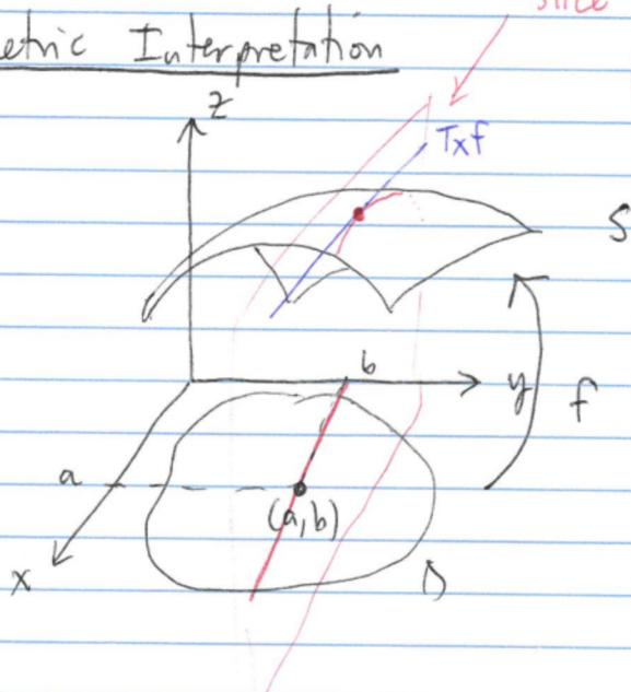
Slice  $y=b$ . The intersection of the plane and the surface is a curve. The partial derivative  $\partial_x f(a,b)$  is the slope of the tangent line to this curve at  $(a,b, f(a,b))$ .
